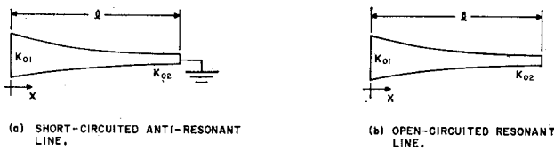
Fig. 1—Types of short- and open-circuited lines required for anti-resonance and resonance, respectively (shown for strip-line).
